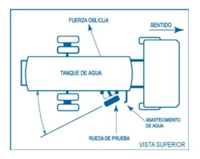
Tests are conducted by pouring water on to the pavement immediately prior to the passage of the measuring wheel, to measure the friction of a wet pavement with a 0.5 - 1 mm sheet of water. Water tanks with capacities ranging from 6,000 to 29,000 I are fitted, depending on the units.
