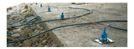
The method generates a vertical profile which gives a graphic view of the depth of foundations, with the reflections caused by upward and downward compression and bending movements. The top or bottom of the structure is struck (horizontally or vertically) and the resulting wave movement is recorded at regular intervals towards the bottom of the foundation element of the structure.
